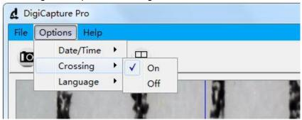
**Noted:** the usage of this crossing is checking the dial on the calibration ruler.
