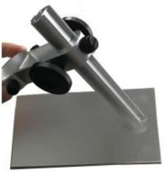
b. Put the microscope into the ring of the stand.
