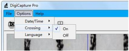
**Noted:** the usage of this crossing is checking the dial on the calibration ruler.
